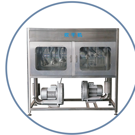
Blower dryer system
